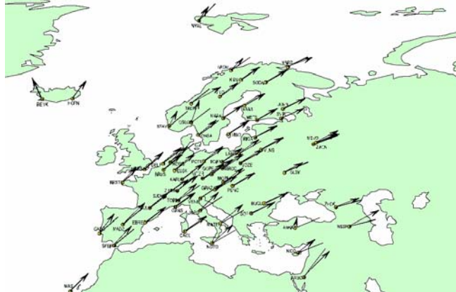
Image 2: Difference between ITRS and ETRS89 due to continental drift
