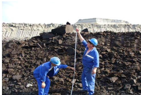
Figure 9 - Measuring the coal layer
